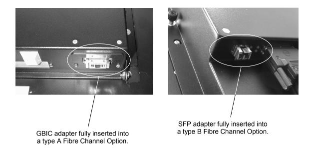
Figure 9-1 Remove the GBIC or SFP Adapter from the Fibre Channel Option
